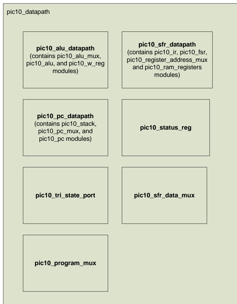
Figure 5. The highest-level Verilog modules inside the pic10_datapath module.
